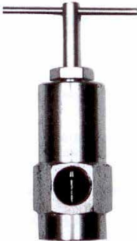
10720 - PRESSURE RELEASING TOOL For use with vent cap fittings and other equipment. Has hardened stem for longer life. 1" - 14 UNS(f) connection, 1/2" NPT(f) thread side port.
