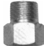
10732 - CONE ADAPTER For adopting vent cop fittings. 1" . 14 UNS(m) X 7/8" . 14 UNF(f) cone. 10594 - 1" . 14 UNS(m) x 3/4"-16 UNF (f) cone. 11177 -1" .14 UNS(m) x 5/8"-16 UNF (f) cone.
