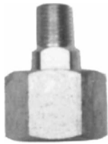
10695 - SCREW CONNECTION COUPLER For servicing vent cap fittings. 1/4" NPT(m) inlet X 1" - 14 UNS(f) outlet. 10715 - 1/4" NPT (m) inlet x 3/4" UNF (f) outlet 10935 - 1/4"NPT(m) inlet x 7/8" -14UNF (f) outlet
