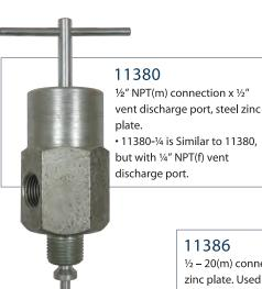
11386  $\frac{1}{2}$  – 20(m) connection, steel zinc plate. Used on Packing Injection Fittings. Relieves excess internal packing pressure, when check ball is forced off seat.
